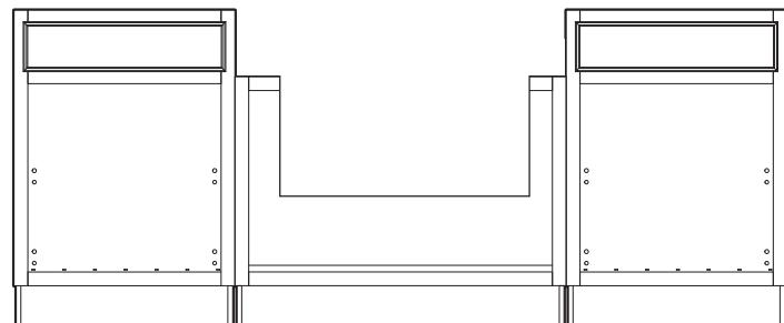
If lower section will remain, fasten to adjacent cabinets (refer to the cabinet installation instructions on the carton or enclosed sheet.)
